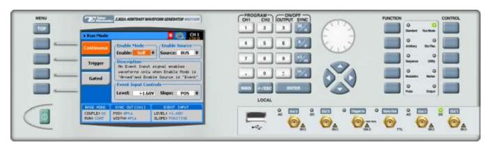
To set a run mode, press the **Run Mode** button in the Control menu.
